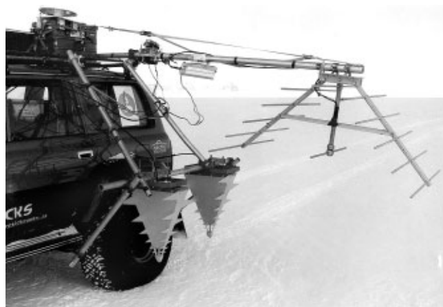
Fig. 3. Antennae configuration on the Toyota Landcruiser for geophysical surveys. The antennas to the right were used for depth soundings (150–160 MHz) and the two close to the vehicle were used for snow radar studies (500–2500 MHz).
