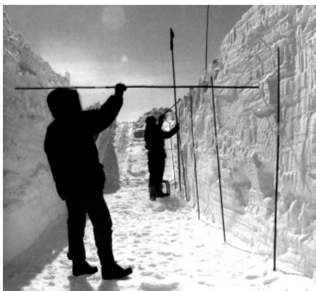
Fig. 2. Mapping of snow layers in a snow pit at Camp Victoria, Amundsenisen.
