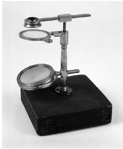
Figure 5.4 An Ellis-type aquatic microscope, similar to the microscope given to Edward Hobson by W. J. Hooker in 1815. Image © Whipple Museum (Wh.1824).
