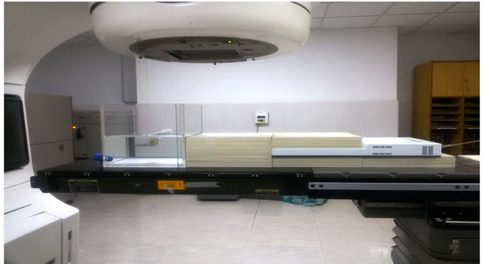
Figure 1. Phantom setup for measurement of the peripheral dose.
