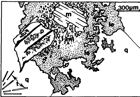
Figure 4. Sketch showing light-grey, quartz-micaceous greisen in the Chanon granite. Primary muscovite (m) is recrystallized into flakes of lithian micas (mi). Biotite is replaced by protolithionites, which occlude needles of rutile. Quartz crystals are invaded by a microcrystalline lepidolitic matrix. t = acicular tourmaline.
