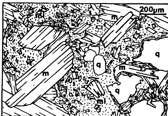
Figure 2. Sketch of light-green, micaceous greisen in albite-muscovite granite. m = large flakes of muscovite and lepidolite; mi = microcrystalline micaceous matrix; q = quartz.
