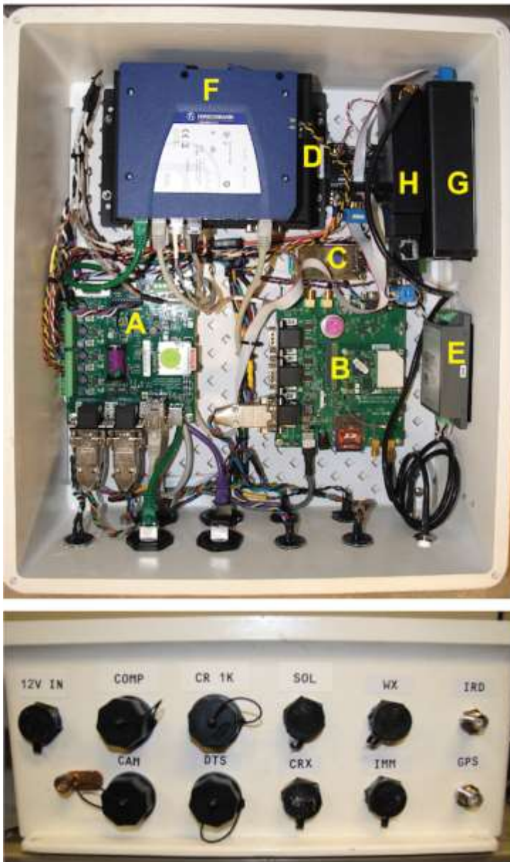
Figure 3. Interior of electronics enclosure box (top) and electronics box connector panel (bottom). Top panel has the major electronic components labeled: A, Triton board from Polar66 Engineering (R. Ross); B, TopCon B110 GPS receiver and carrier board; C, SeaBird Inductive Modem Module (IMM) for decoding inductive data transmission from the ocean sensors; D, WinSystems Windows-OS computer for interfacing with the DTS controller; E, a power regulator to provide 12.0 volts to the PTZ camera; F, ethernet hub; G, dial-up router; H, NAL AL3A-R Iridium modem. The white electronics enclosure box is 40 x 30 X 25 cm. Lower panel is an image of the exterior bottom wall of the enclosure, showing the port arrangements for the AMIGOS-3. Port functions clockwise from upper left: power, ethernet access (for operator), Campbell Scientific CR-1000X ethernet, four-wire input for albedometer, five-wire input for Vaisala weather data and sensor power; two-wire input from Seabird inductive coupler circuit (ICC) to IMM; three-wire power input to the CR-1000X; DTS ethernet; camera ethernet (with power-over-ethernet); grounding lug.
