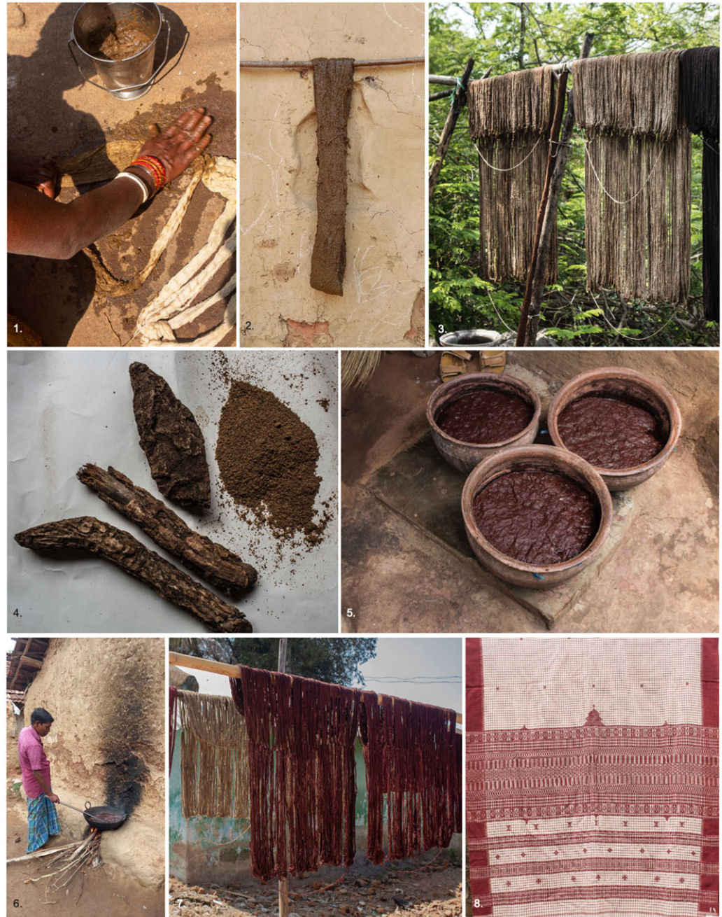
Figure 2. Clockwise from left, Pic 1: Application of cow dung, castor oil, and ash water as part of the yarn preparation process. Pic 2: Hanging the yarns coated with cow dung for the biodigestion process. Pic 3: The change in colors of the yarns after one month of repeating the same process and drying them under the sun. Pic 4: The root skins of Morinda citrifolia trees (Aul) used for dyeing. Pic 5: Soaking yarns in Aul dye, castor oil, and ash water, and tanning for one day under the sun before boiling the yarns. Pic 6: Boiling the yarns in big iron vats by the weaver. Pic 7: Drying the dyed yarns under the sun. Pic 8: The usage of Aul-dyed yarns in a traditional Kotpad saree woven by Kapileshwar Mohanto.
