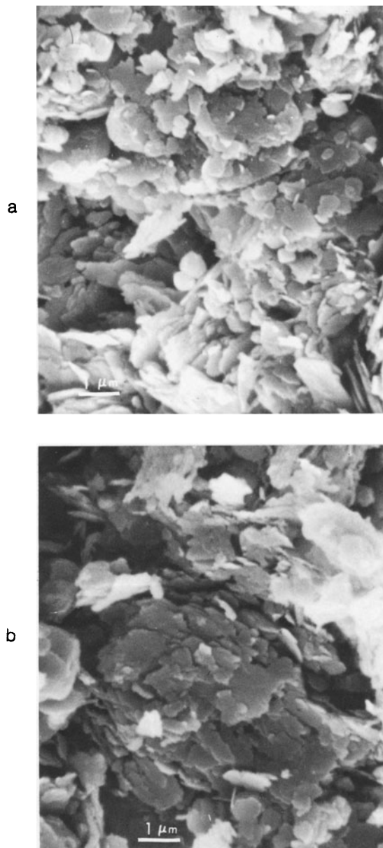
Figure 4. Scanning electron micrographs of Ashland kaolinite showing a lack of texture and the irregular outlines of individual etched grains.
