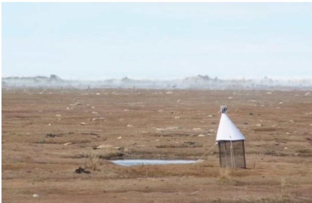
Figure 2. Photograph of International Polar Year (IPY) trap set on the coast of Akimiski Island, Nunavut, Canada. The pitfall portion of this trap is set below the interception screen at ground level. The white cone acts as a rain shield to prevent the pitfall trough from filling with rainwater and as a funnel to direct climbing insects up into the collection head at the top. Photo by Lisa Pollock.
