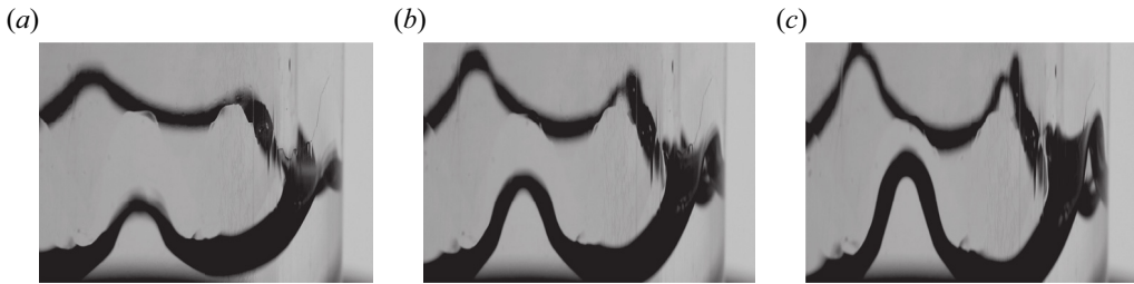
Figure 13. These three snapshots correspond to snapshots (b–d) of figure 12 and show, using a different light contrast, how the contact line constantly moves over a wetted substrate due to the presence of a stable thin film deposited and alimented at each cycle.
