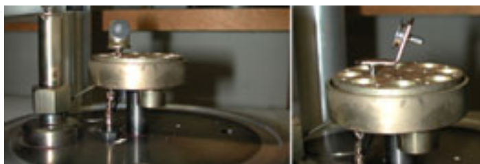
Figure 1 (left). End face view of SEM stub in modified shelf bracket, in sputter coater.
