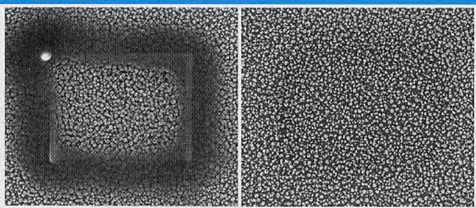
A silicon "grass" sample irradiated for 10 minutes before (left) and after (right) the use of Evactron SEM-CLEAN device. 50kX -From Active Monitoring and Control of Electron Beam Induced Contamination by Andras E. Vladar, Michael T. Postek and Ronald Vane\* "Active Monitoring and Control of Electron Beam Induced Contamination" Proc. SPIE Vol. 4344 (2001), 835
