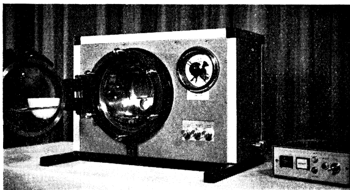
High Pressure Oxygen Combustion Unit
