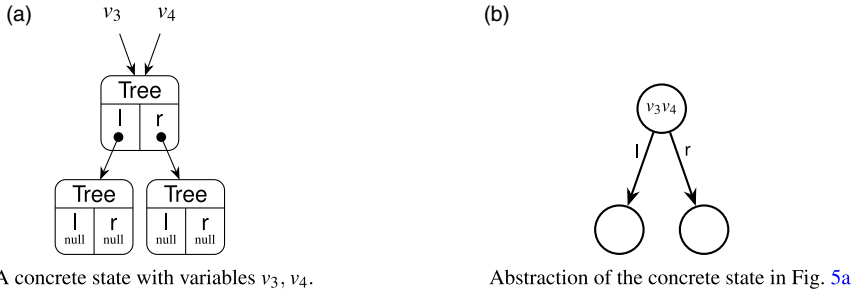
Figure 5. Concrete and abstract states illustrating aliasing.
