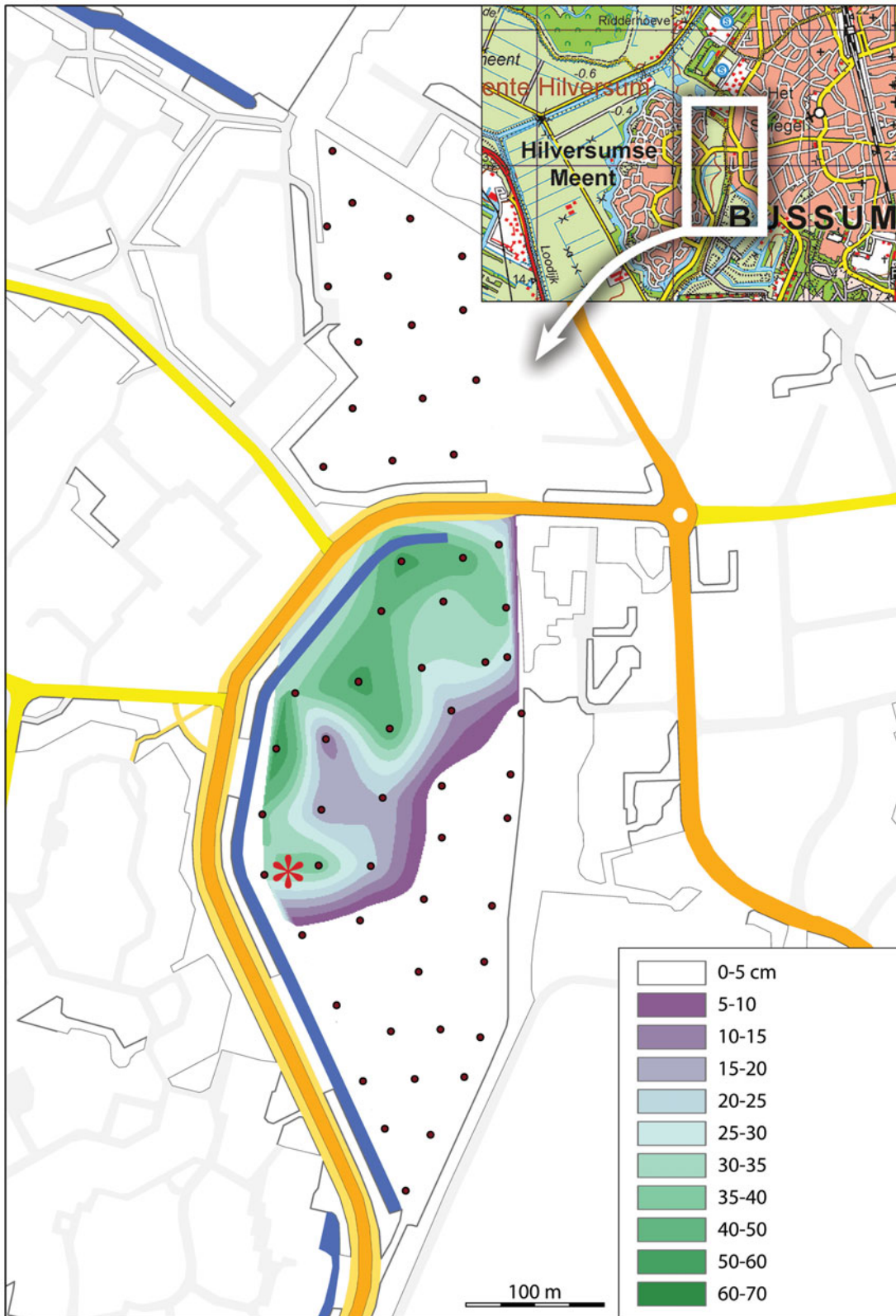
Fig. 2. Map showing the occurrence and thickness of the peat deposit, based on linear interpolation. The sampling location is indicated by * and corings are indicated by black dots.
