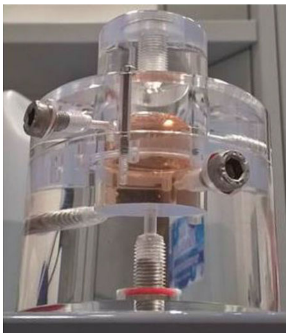
Fig. 5. Membrane testing for system B. The testing of the flexible membrane for prototype B being carried out at Kayser Italia. This test demonstrated that very little pressure was required in order to cause the membrane to flip inside out.
