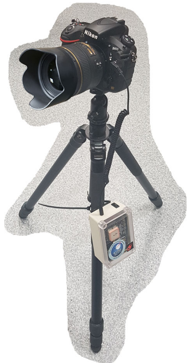
Figure 1. One of the observatories used in the OSIRIS-REx observation campaign, complete with the custom-designed triggering unit.
