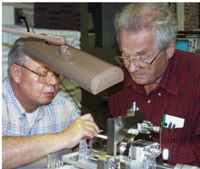
Figure 4: Samuel N. Jones of NIST and Oliver C. Wells preparing a sample for viewing on the modified specimen stage of the NIST high-resolution field emission SEM. The modified stage held both the LLE detector and the sample.
