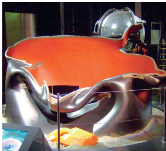
One of six bracings supporting the Alexander L. Kielland, a Norwegian oil rig that failed in 1980 from a fatigue crack resulting from a poor weld. Of 212 people aboard, only 89 survived the accident. This section of the rig is on display at the Norwegian Petroleum Museum in Stavanger. ©2007 Jarle Vines, some rights reserved.
