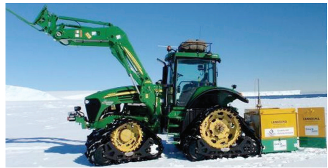
Fig. 7. Rate-controlled CPT (20 mm s -1 ) in Antarctic multi-year fast ice to depths exceeding 1 m using standard equipment (McCallum, 2012).
