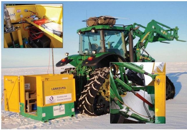
Fig. 2. CPT operating 'box' fitted to a BAS tractor, configured ready for use. Insets show rigid link installed and data-collection equipment.
