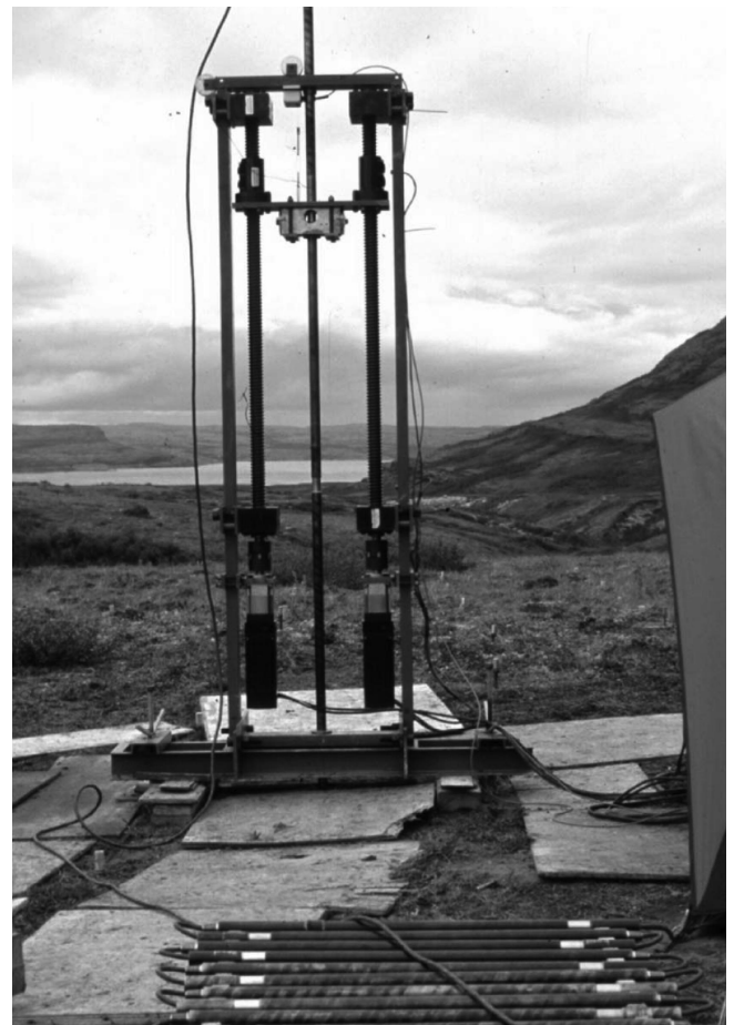
Fig. 5. Linear pushing system for rate-controlled CPT. (From Bateau and others, 2005, Rate-controlled cone penetration tests in permafrost, Can. Geotech. J. , 42 (1), figure 2 © 2008 Canadian Science Publishing or its licensors. Reproduced with permission.)
