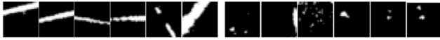
Figure 4. Examples of positive fireball samples (left group of six images) and negative samples (right) for neural network training.
