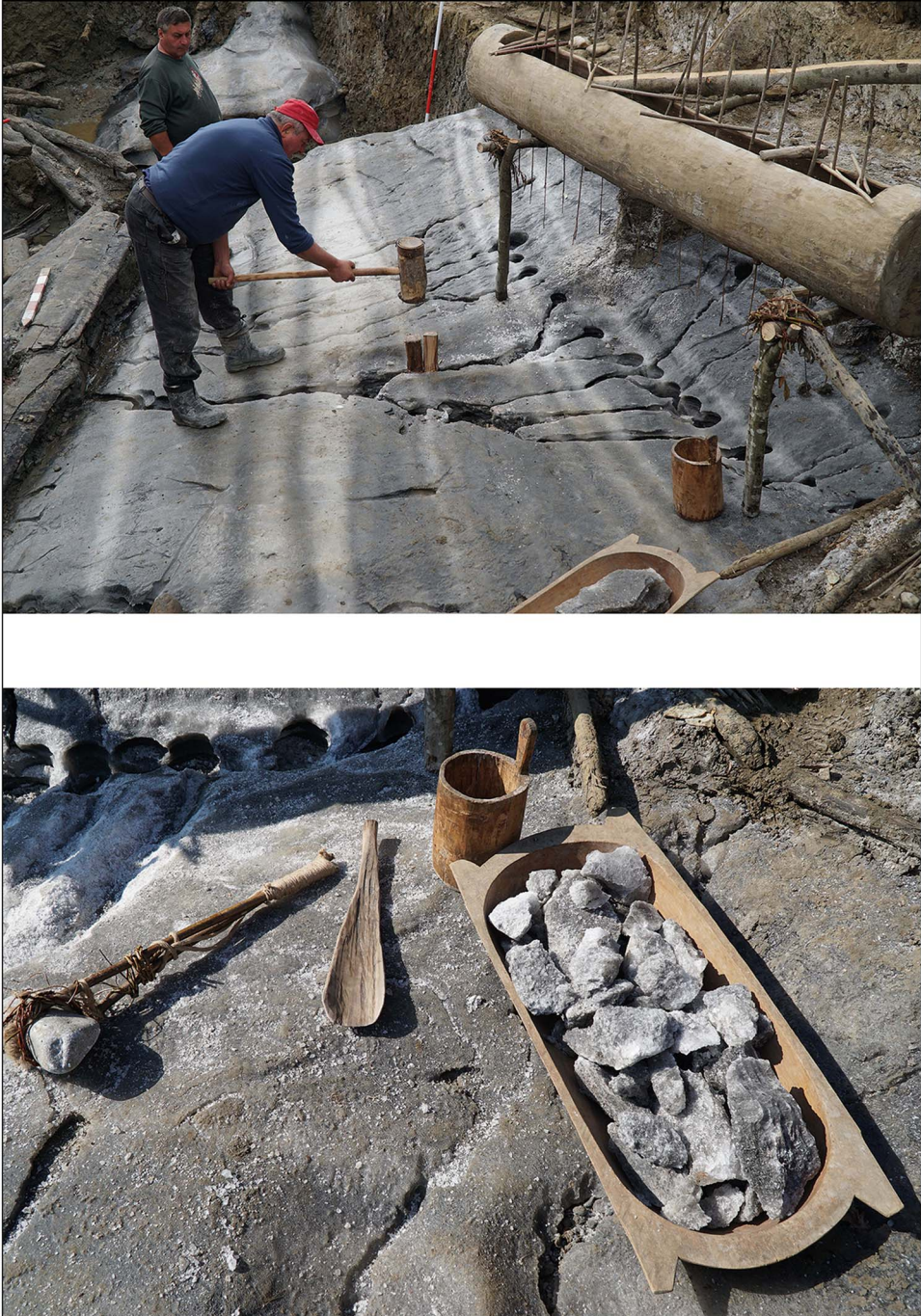
Figure 9. Top) hammering wedges into the channels formed; bottom) tools used in the experiment (bucket, hafted stone hammer, scoop), and the rock salt collected (figure courtesy of the National Museum of the Eastern Carpathians).
