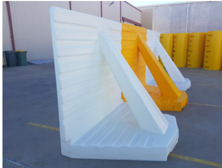
FIGURE 2. The EP prototype units. The main features are evident: a square vertical face with a horizontal base and a support strut. On site the shell is filled with a suitable material.
