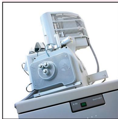
dispersive X-ray spectrometers (EDS) to automatically acquire image and composition information from a large number of samples—typically polished sections of particulates from mineral processing operations and drill core, or lump materials from exploration. More information can be found at: [www.fei.com](http://www.fei.com).
