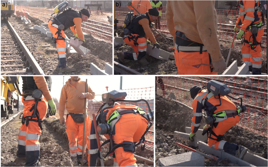
Figure 6. Testing of the in-field operational setup during which conduit module TT3135 weighing 30 kg was handled to perform (a-b) Gross Positioning (GP) task, and (c-d) Fine Positioning (FP) task.
