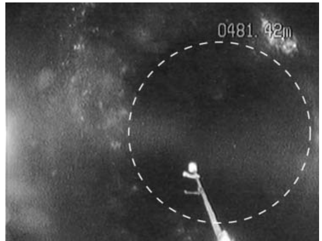
Fig. 14. Indistinct exit cavity in the 'honeycomb' ice at the borehole base, as captured by the down-looking camera.
