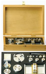
Designed for a multi-instrument environment, the EM-Tec U2 universal SEM sample holder and SEM stub adapter kit will hold a wide variety of SEM samples, up to a diameter of 42 mm. Samples can be flat, round, block, or oddly shaped. Included in this kit is a useful selection of SEM stub adapters, which enables using the kit on virtually any SEM. Holders are fully compatible with FEI/Philips, JEOL, Hitachi, Tescan, Zeiss/LEO, and other brands of SEMs.
