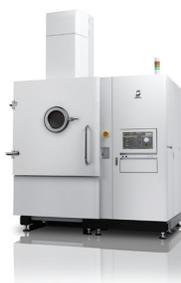
JEOL provides technology leadership in both electron microscopy and e-beam lithography with new Additive Manufacturing technology for 3D printing. The company has introduced a new PBF-style EBM system, the JAM-5200EBM, which significantly improves quality and manufacturing time to produce stronger and lighter parts for a variety of applications. Benefits include a cathode life of over 1,500 hours, a clean, helium-free environment, and JEOL's extensive service network.
