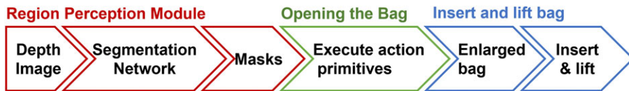
Figure 3. Pipeline for our method: The perception module takes depth images and outputs segmentation masks for the bag handles and rim. The robot grasps the key points and executes dynamic actions. Last, the robot inserts the items and lifts the bag.
