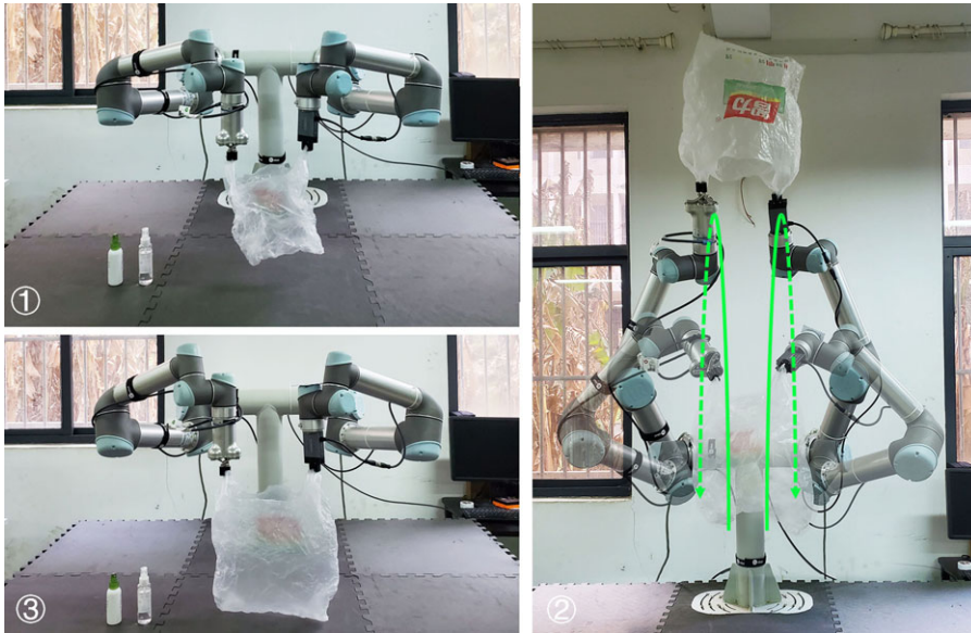
Figure 7. Dual-arm Shaking: (1) Preparation for dynamic dual-arm shaking. (2) Long-distance and high-speed shaking. (3) An enlarged bag.
