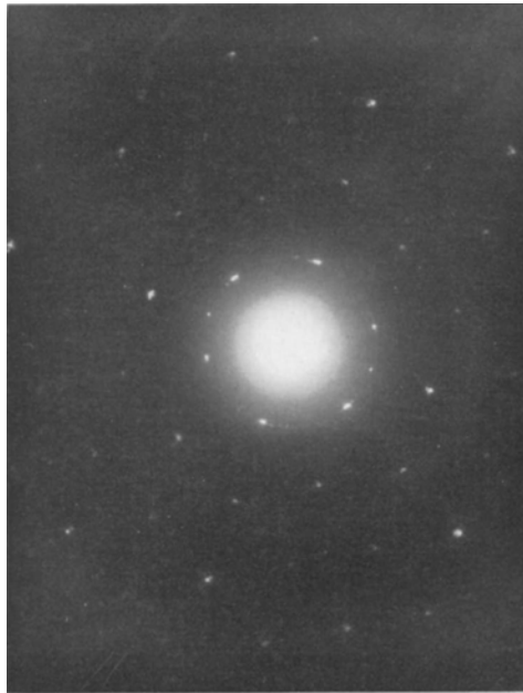
PLATE 10. Selected area electron diffraction pattern of a sixfold mica star growing symmetrically on a kaolinite crystal core from the St. Peter sandstone. The six brightest inner spots are the three pairs of (020) spots contributed by the three mica needles. There is a single pair of weak spots at the same radius corresponding to the (020) of the kaolinite, rotated 30^\circ from those of the mica (020). For a defocused image of same cluster see Plate 11. Note evidence that all grains are lying on their (001) as there are no inner spots larger than the 4.50 \text{ \AA} of the (020).
