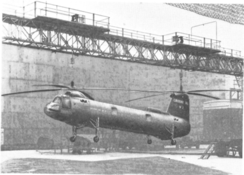
by Courtesy of Bristol Aircraft Ltd Fig 3 Bristol 192 on gantry rig
