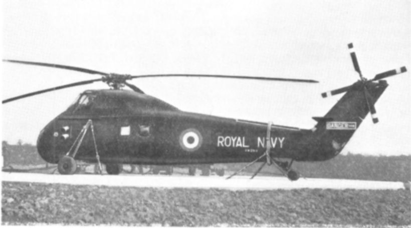
Fig 4 Wessex tethered for ground running
