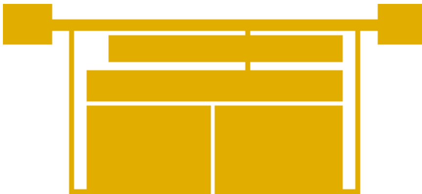
Fig. 9. The proposed power divider's layout.
