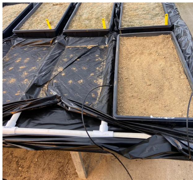
Figure 2. Greenhouse design for preemergence dose-response screening studies. Each flat filled with soil was placed in an individual cell for subirrigation to prevent herbicide contamination between flats from water movement.
