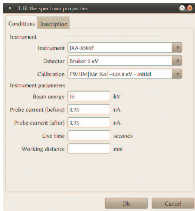
Figure 2: The spectrum properties dialog . This dialog permits editing the properties of one or more spectra.
