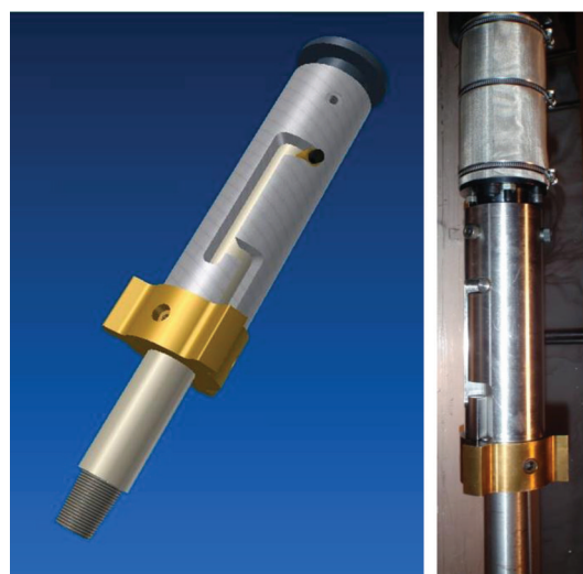
Fig. 7. Bayoneted coupling between the pump section and extension rods of the adapted rock drill. The pump section at the top of the right photo is covered in a fine-mesh filter that was replaced after each run when it became coated in sediment particles. The extension rods threaded onto the lower part of the bayonet coupling. The bayonet could be used to provide a hammer effect when making a hard-core break, or be released if the drill head was stuck, thus recovering all of the upper parts of the drill sonde. Fortunately this never needed to be used in the rock drilling at NEEM.
