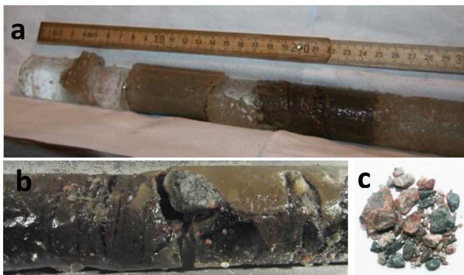
Fig. 9. Cores from the rock drill with (a) banded glacial ice and sediments and (b) an ice/rock mix, including pebble-sized stones, and (c) an assortment of stones from the rock cores.
