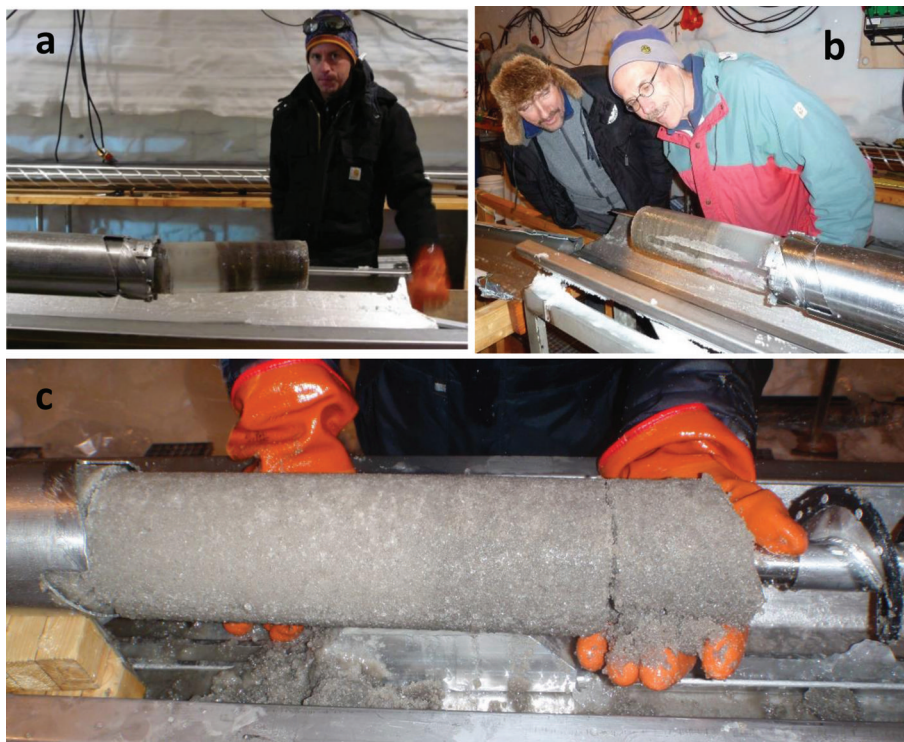
Fig. 1. The final cores collected at NEEM approaching the obstructions at 2537.36 and 2538.10 m depth were drilled with the Hans Tausen drill mounted on the NEEM deep-drill electronics, motor and gear sections. Banding silty and sediment-laden ice can be seen in (a, b). The chips also contained sediment material (c). The cores pictured were collected in 2011 with ice cutters with carbide inserts (Fig. 4). Similar cores with standard ice cutters were obtained to close the 2010 season.
