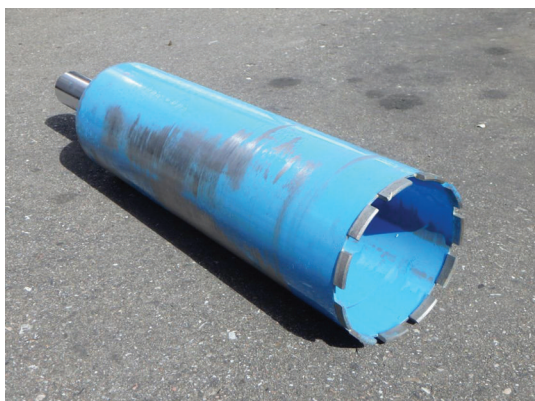
Fig. 10. Concrete diamond core bit with threaded attachment to mount to rock-drill extension rods and bayonetted connection to the pump section. This head was attached to the rock-drill extension rods, and ultimately dislodged the stone obstruction at 2538.1 m.
