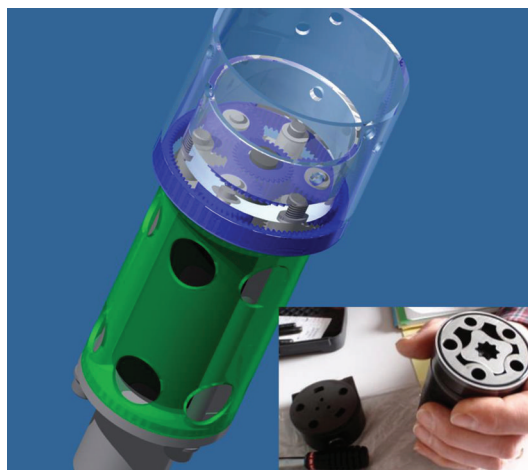
Fig. 6. The pump and gear section for the adapted rock drill. The upper part of the gear section is constructed to be mounted onto the rotating bearing at the lower end of the deep-drill motor and gear section, which, in turn, turns pump gear (blue) and the hydraulic pump (internal mechanism view shown inset at lower right) which is housed inside the green section. Depending on the orientation at which it is mounted, the flow direction can be reversed. With the speed of the outer toothed wheel set by the drill motor, the pump gear was designed to turn three times as fast as the rotating drill shaft. The large holes in the green section are lined with a fine-mesh filter to protect the pump from the rock dust and sediment produced during cutting while allowing liquid to flow through the pump.
