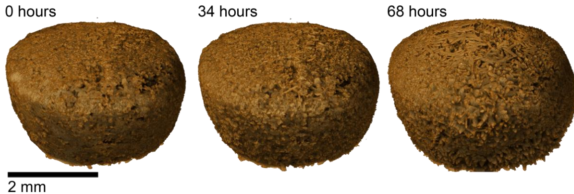
Figure 1. 3 time steps out of 138 full X-ray microtomography datasets that show the formation of gypsum crystals on the Lede stone.
