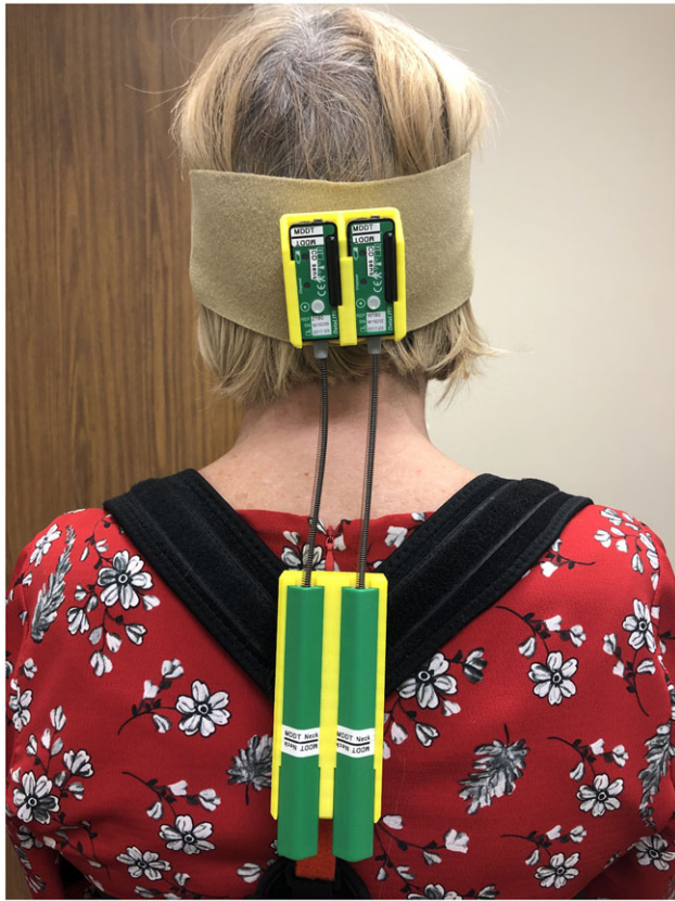
Figure 2. Depiction of the placement of the torsiometer and goniometer sensors for kinematic cervical dystonia assessment.
