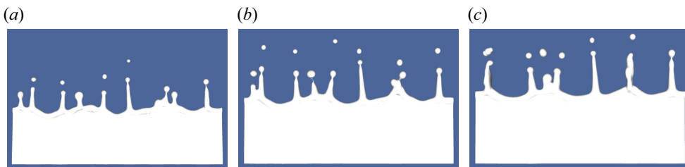
Figure 12. Snapshots taken from a simulation case at We = 160 , \varepsilon = 0.04 and N_{max} = 25 showing ligaments merging on the corrugated rim bordering the expanding sheet, while shedding fragments via the end-pinching mechanism. From left to right: t/\tau_{cap} = 0.73, 1.09, 1.45 .
