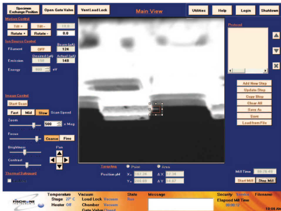
Figure 2: 900 eV secondary electron image of a lamella acquired at 10° stage tilt.
