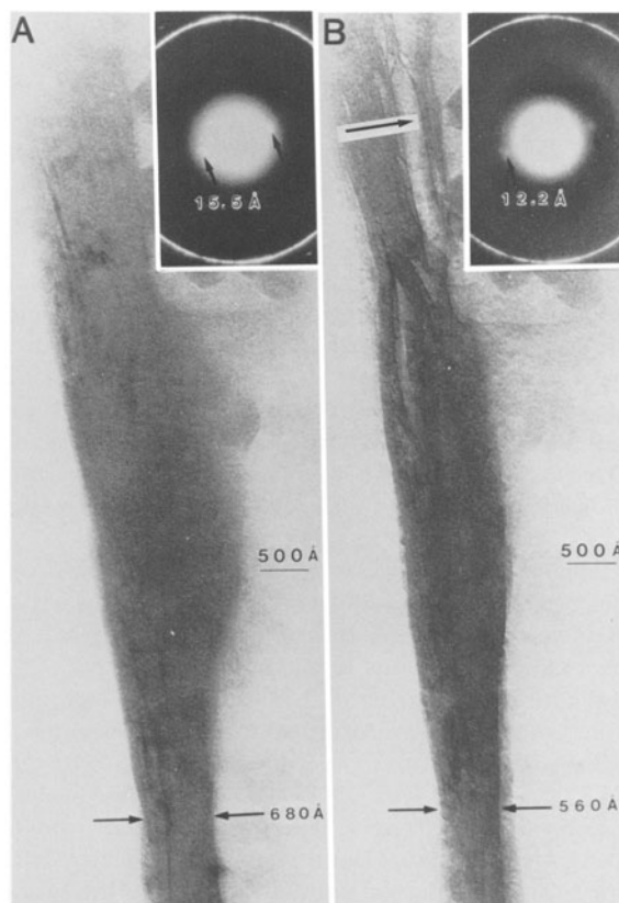
Figure 5. Humidity-controlled transmission electron micrographs of hydrated Na-smectite (A) in a humid-air environment at 60 Torr and (B) the same particle in a dry-air environment at 50 Torr, after evacuation for 1 hr at 25–70°C. Micrographs show differences in morphology and of interlayer spacing and presence of aerosol-size fine particles produced by air-drying (arrow).
