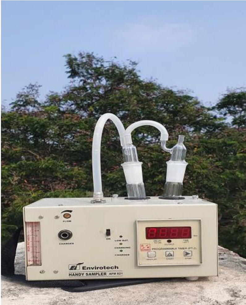
Figure 2 Handheld air sampler used for bubbling air sample through NaOH solution.
