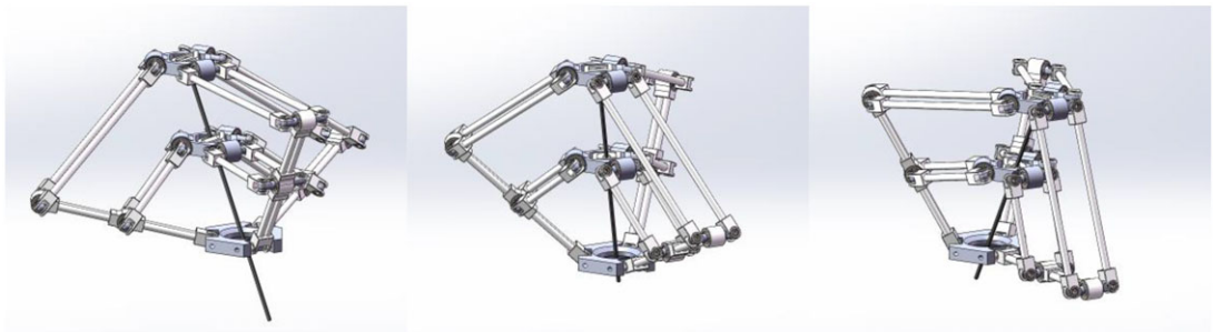
Figure 9. Different configurations of the mechanism with the given positions in Table II.
