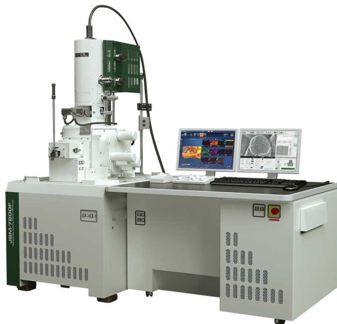
Figure 1: The JEOL JSM-7800F analytical SEM requires low floor vibrations and low electromagnetic fields in order to perform at its highest performance levels. Image courtesy of JEOL USA, Peabody, USA.
