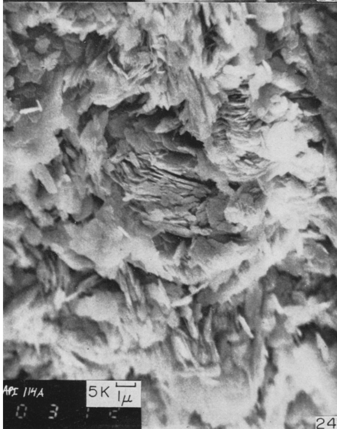
Fig. 23. Cornwall kaolin, Imperial Pit. 3000× (0011).
