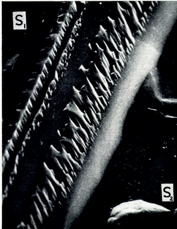
Fig. 4. Detail of etch pits formed on the side wall of hexagon indicated by the large circle in Figure 1. ( \times 1000 .)
