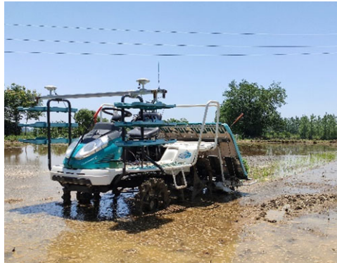
Figure 13. The field experiment of automatic operation of rice transplanter.
