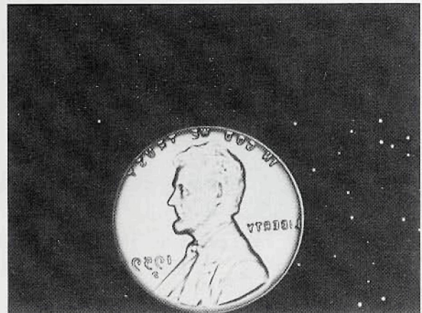
Figure 1: Acoustical image taken at 30 MHz of a 1959 penny with backside shaved. White dots in background represent air bubbles. Reflections from top and bottom surfaces were gated in to produce this image.
