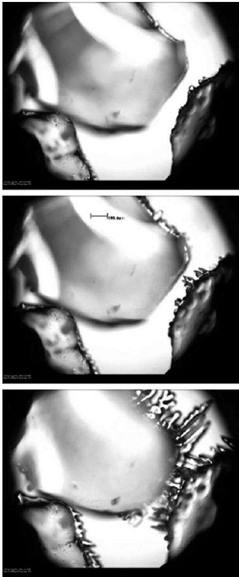
Fig. 1. This top-to-bottom sequence of images demonstrates the development of solid columnar dendrites that were observed at -5^{\circ}\text{C} . c -axis growth is dominant at this temperature. Protrusions develop only on specific surfaces of the original ice crystals. The growth from the lower right eventually joined with the crystal that occupies the center space in the images. There is neither measurable sublimation nor growth from this surface. Time lapse between the first two images is 20 min and from the middle to the bottom is 1 hour 56 min. The image sequence was begun when this feature of interest was located: \approx 20\text{--}30 min.
