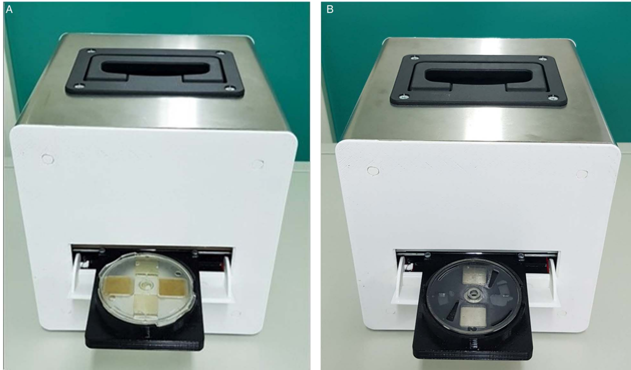
Fig. 1. KFM used with the Mini-FLOTAC (A) and FLOTAC devices (B).
