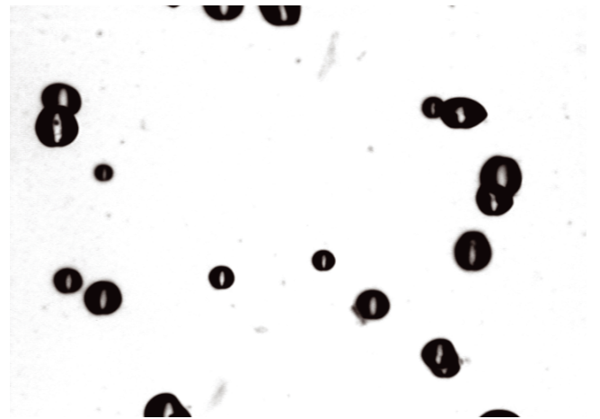
Fig. 1. Thick-section image taken with a large depth of field, showing all air bubbles in the sample volume. This micrograph shows several clusters of two overlapping bubble images, created by bubbles at different depths inside the sample.
