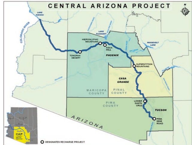
Figure 4. Map of the CAP that provides water supplies to central/southern Arizona from the Colorado River, whose flow levels are dependent upon snow pack and precipitation in the entire Colorado River Basin. The CAP pumps water uphill over 320 miles to the Phoenix and Tucson metropolitan areas, and to agricultural and Native American communities in between, with a total elevation gain of approximately 1600 ft (from Ref. 47: http://www.cap-az.com/about-us/system-map ).
