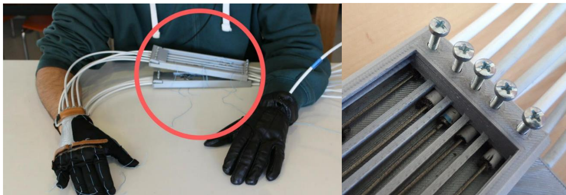
Figure 9. Calibration system (red circle) and a detail of the adjustment system on the right.
